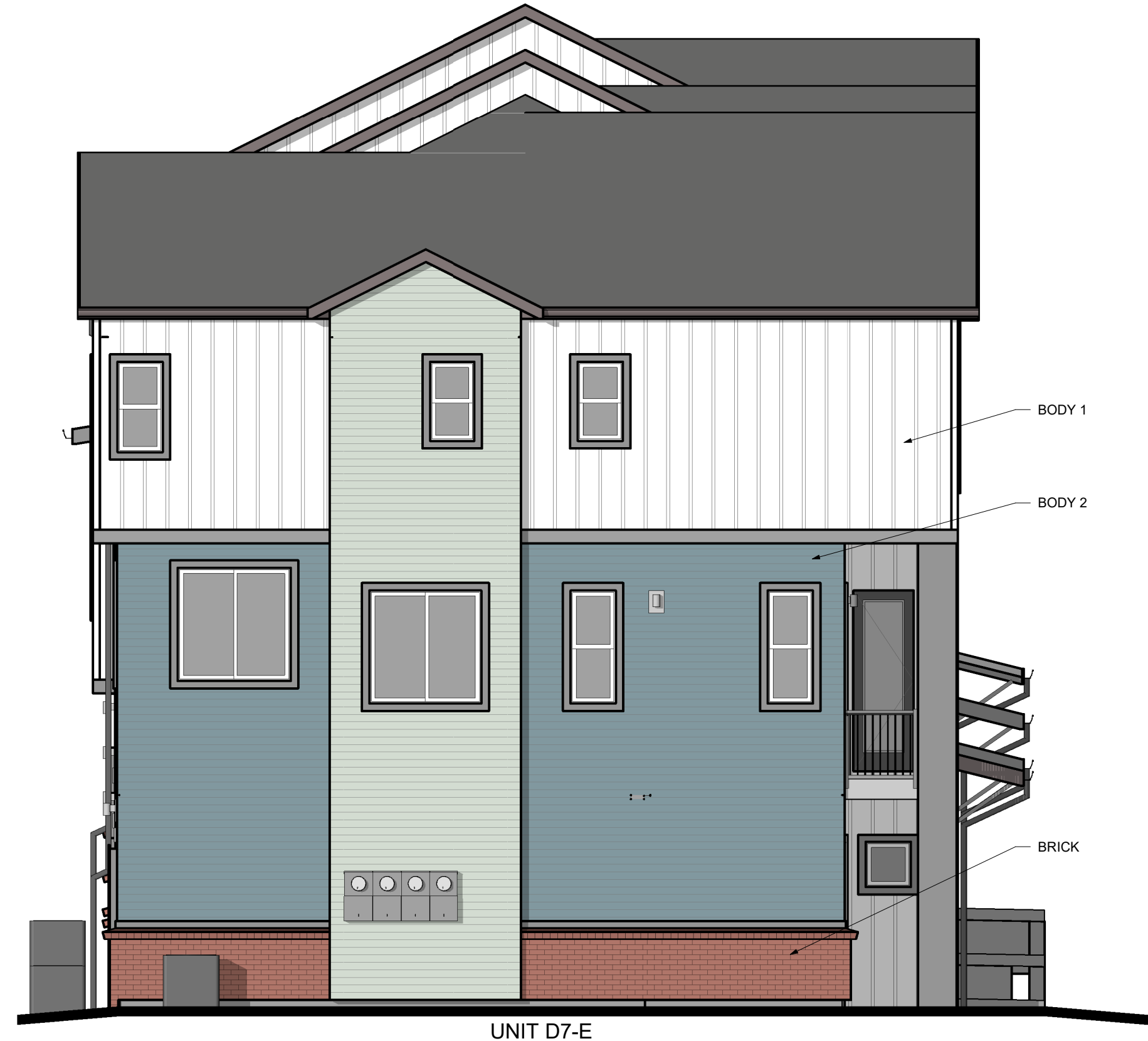
2 BUILDING 4 - LOTS 19-22 - 4-PLEX - SIDE ELEVATION 3/16" = 1'-0"
