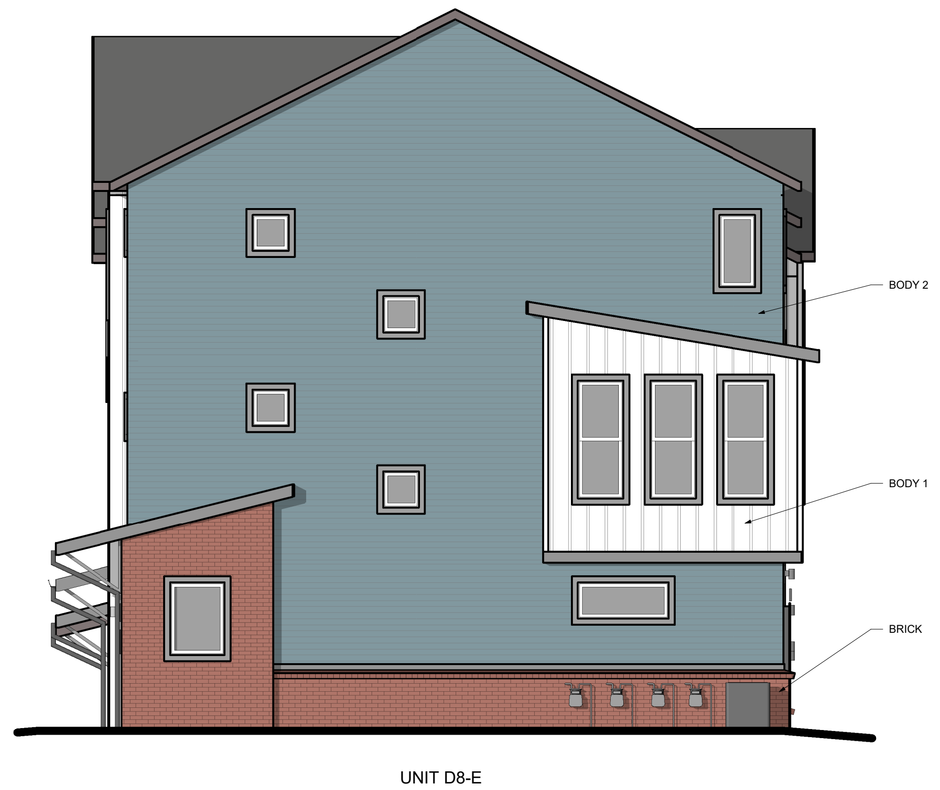
1 BUILDING 4 - LOTS 19-22 - 4-PLEX - SIDE ELEVATION 3/16" = 1'-0"
