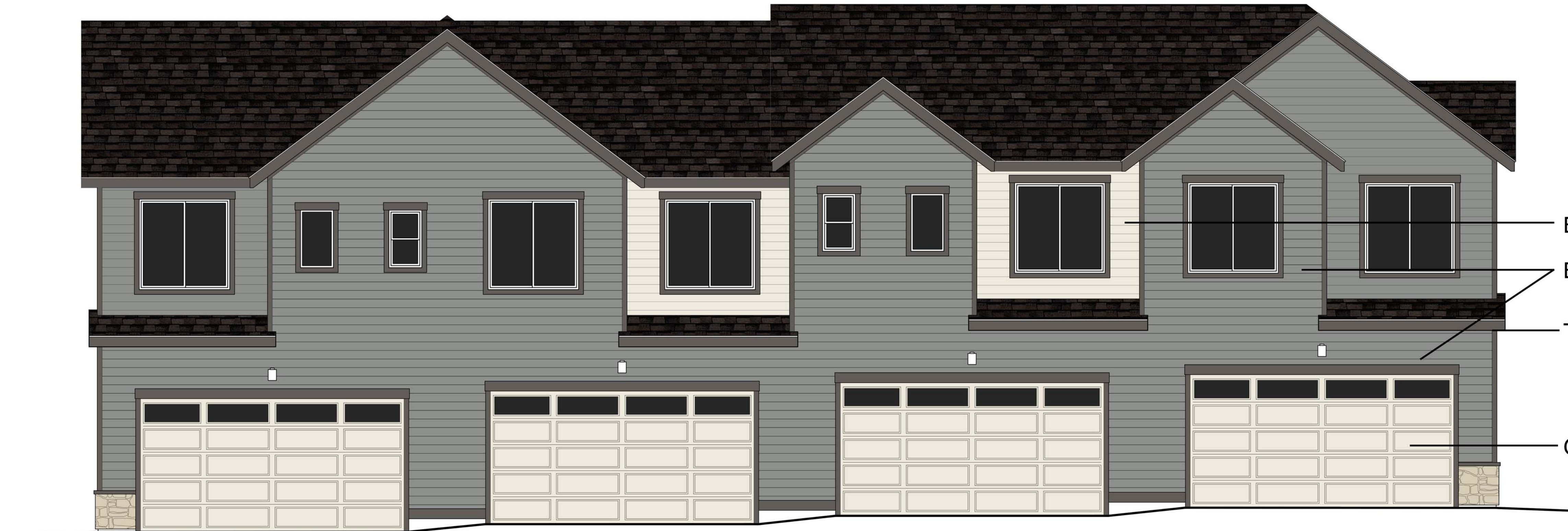
1 BUILDING 1 - LOTS 1-4 - 4-PLEX FRONT ELEVATION SCALE: 1/4" = 1'-0"
