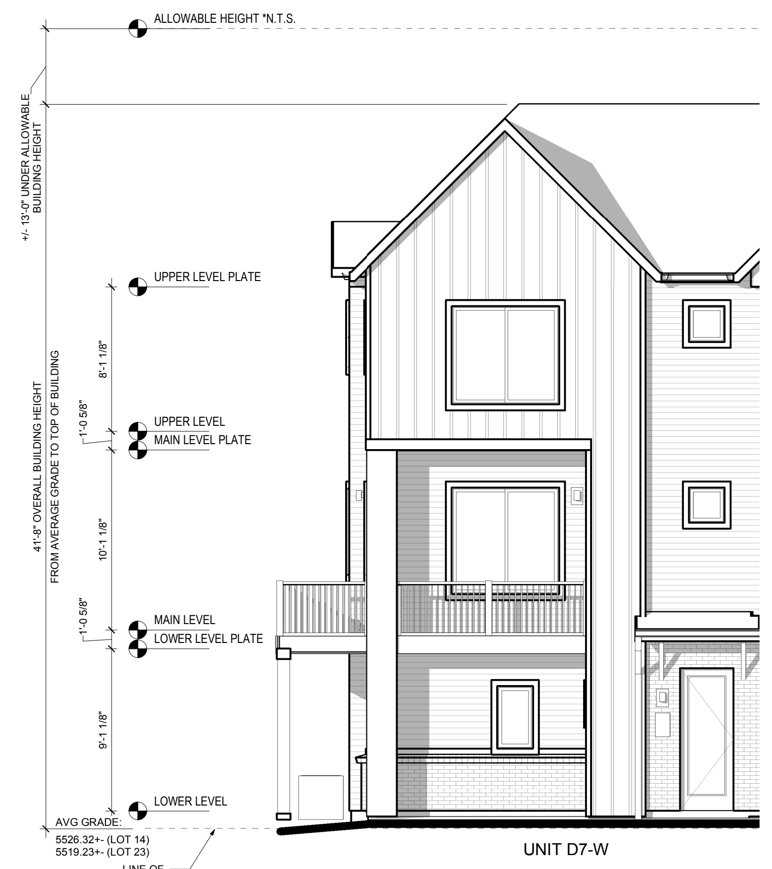
3 3-PLEX - FRONT ELEVATION W/ DECK WRAP (LOTS 14 & 23) 3/16" = 1'-0"
