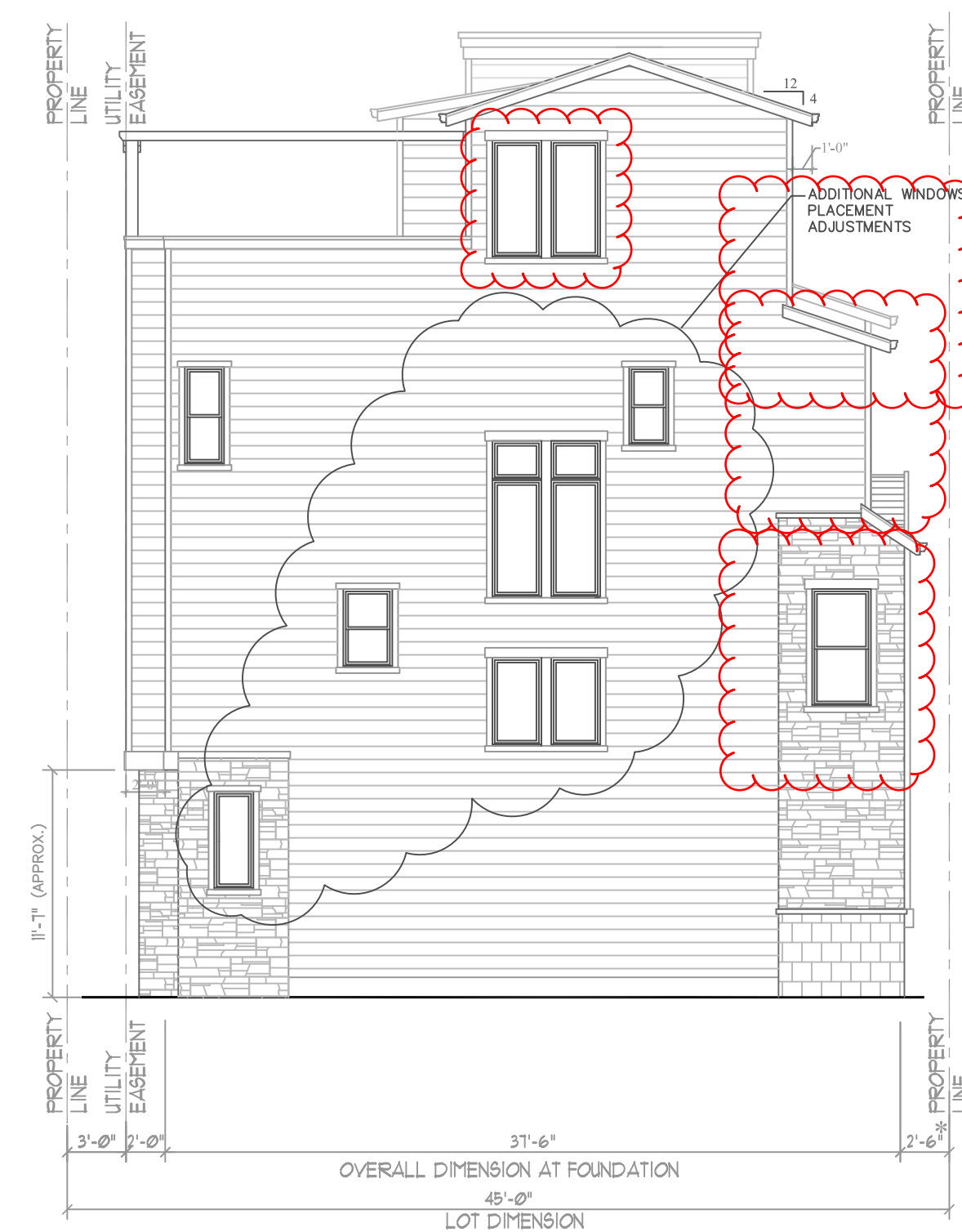
LEFT ELEVATION 'B' 802 PLAN 1/8"=1'-0" ALL LAP SIDING TO BE CEMENTITIOUS 4-STORY OPTION
