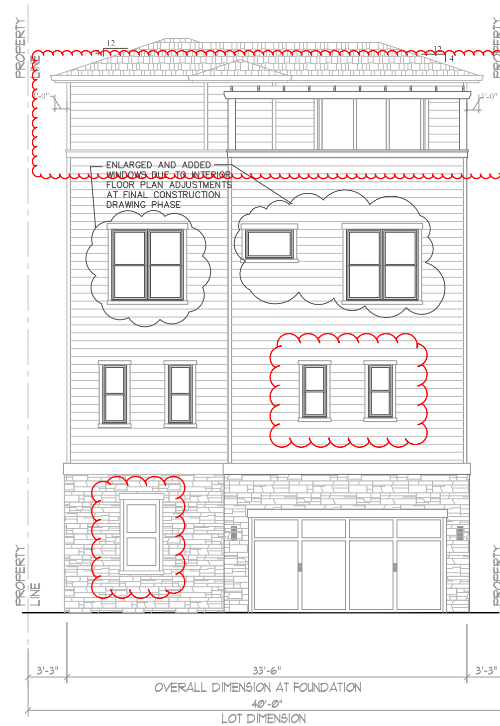
REAR ELEVATION 'A' 802 PLAN 1/8"=1'-0" ALL LAP SIDING TO BE CEMENTITIOUS 4-STORY OPTION
