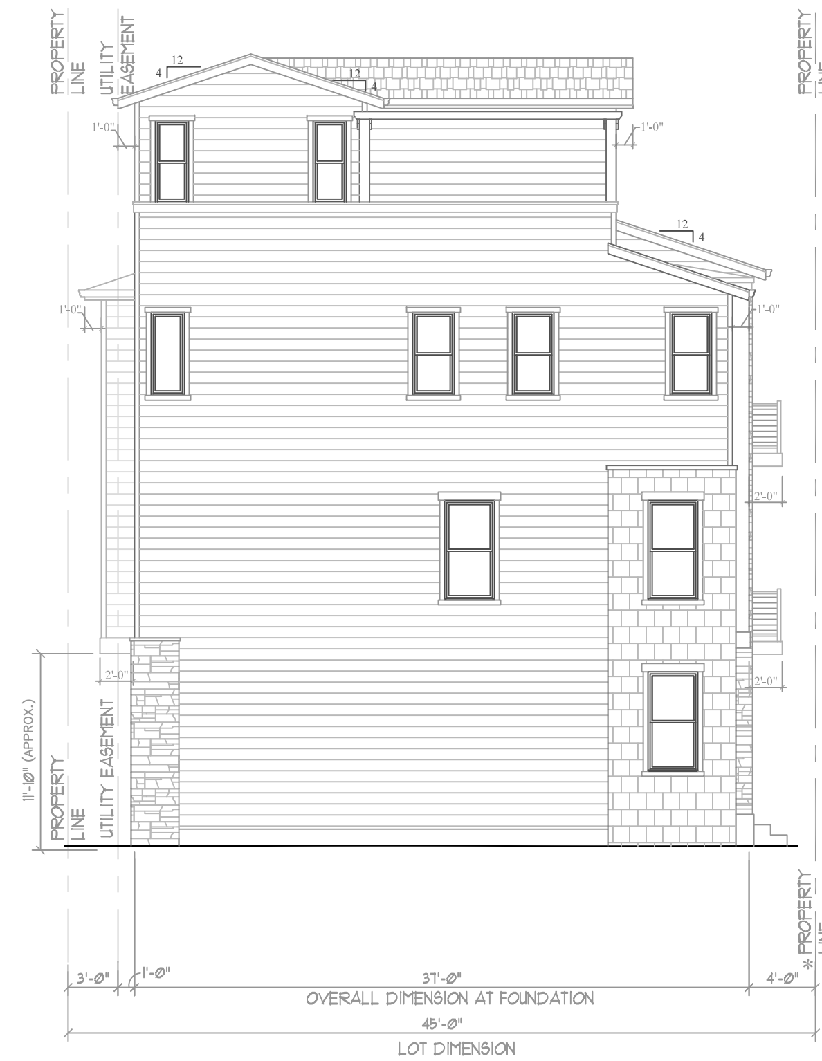
LEFT ELEVATION 'B' 803 PLAN 1/8"=1'-0" ALL LAP SIDING TO BE CEMENTITIOUS 4-STORY OPTION
