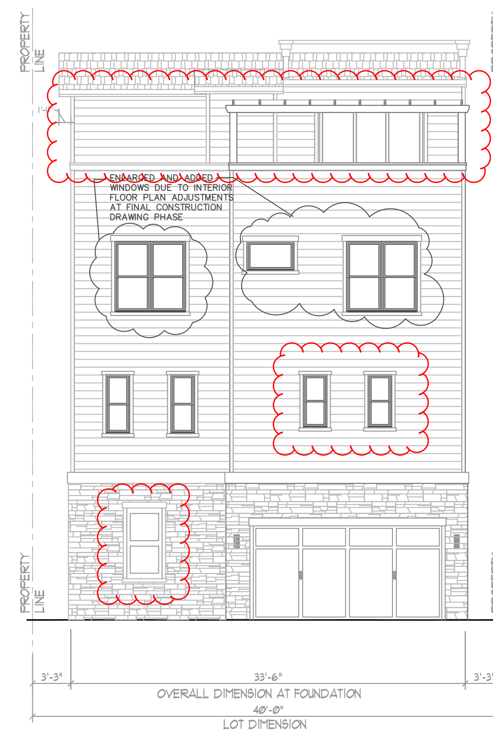
REAR ELEVATION 'B' 802 PLAN 1/8"=1'-0" ALL LAP SIDING TO BE CEMENTITIOUS 4-STORY OPTION
