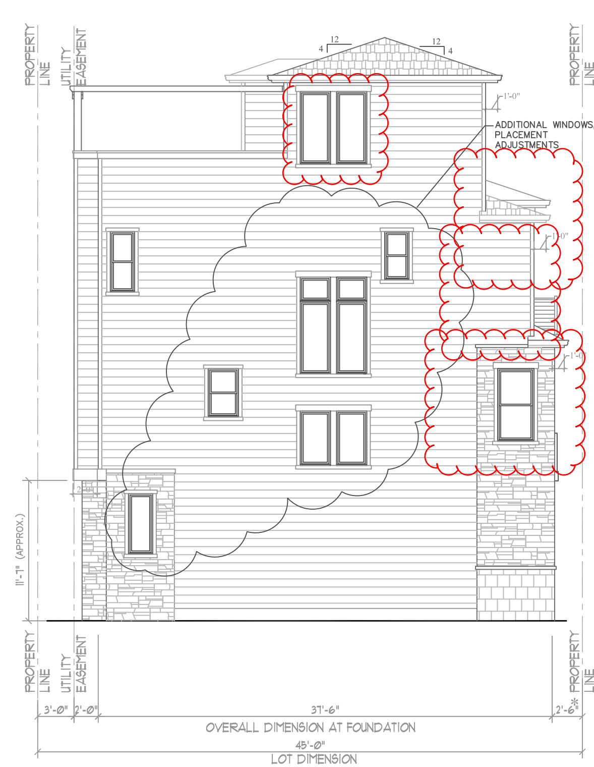
LEFT ELEVATION 'A' 802 PLAN 1/8"=1'-0" ALL LAP SIDING TO BE CEMENTITIOUS 4-STORY OPTION
