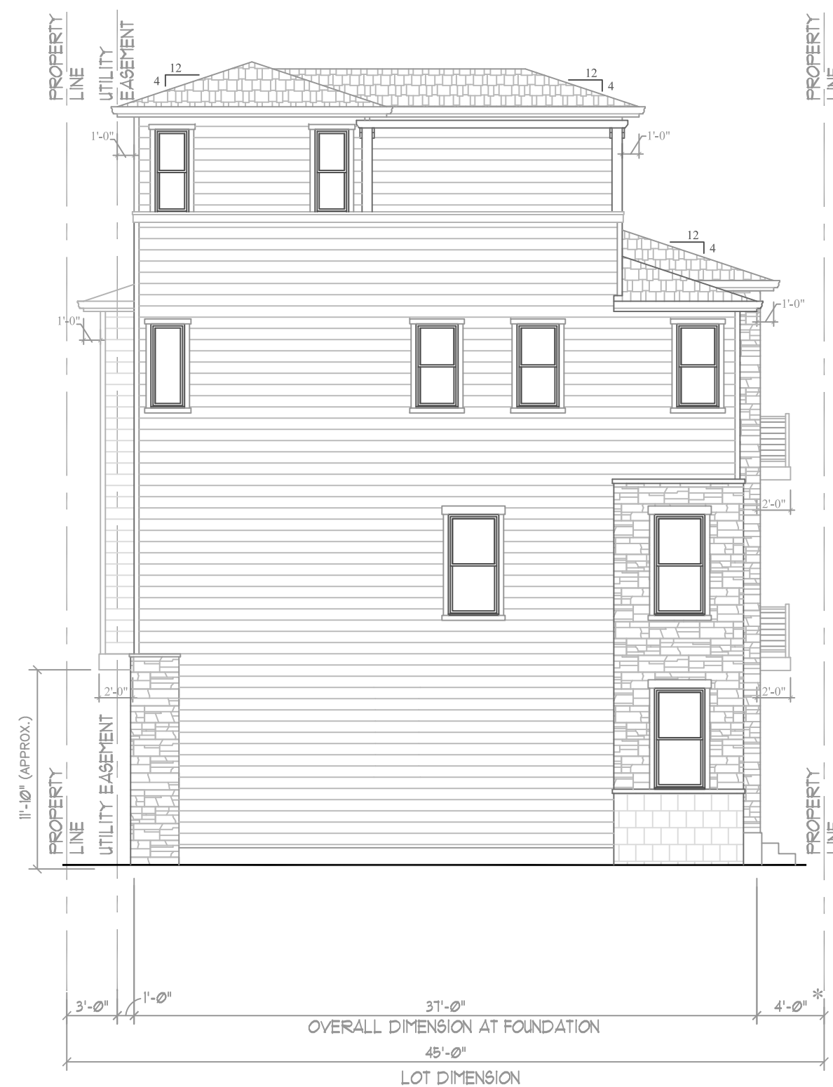
LEFT ELEVATION 'A' 803 PLAN 1/8"=1'-0" ALL LAP SIDING TO BE CEMENTITIOUS 4-STORY OPTION
